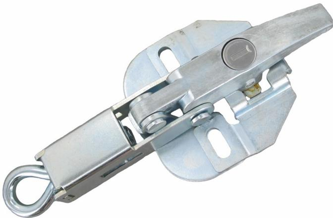
This simple lever operated compression hook latch provides a secure over-center action and the spring-loaded eye-hook incorporates tension to keep panels rattle free and secure. Designed for applications where the latch and keeper are surface mounted on the same plane, folding the robust lever down pulls mating in-line panels tight.
